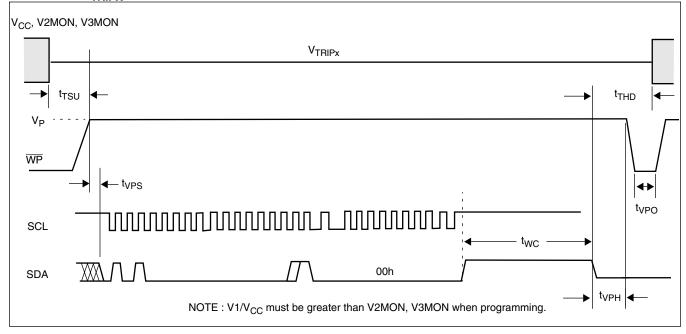
Figure 34. DCP "Wiper Position" Timing
