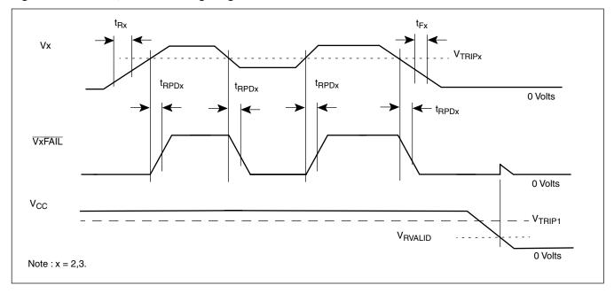
Figure 33. V<sub>TRIPX</sub> Programming Timing Diagram (x=1,2,3).
