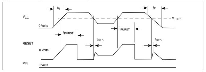
Figure 31. Manual Reset Timing Diagram
