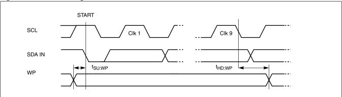
Figure 29. Write Cycle Timing
