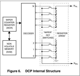
At both ends of each array and between each resistor segment there is a CMOS switch connected between the resistor array and the wiper  $(R_{Wx})$  output. Within each individual array, only one switch may be turned on at any one time. These switches are controlled by the Wiper Counter Register (WCR) (See Figure 6). The WCR is a volatile register.
