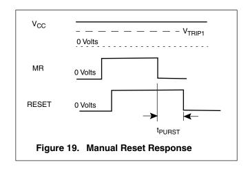
RESET remains HIGH for time t<sub>PURST</sub> after MR has returned to its LOW state (See Figure 19). An external "pull down" resistor is required to hold this pin (normally) LOW.
