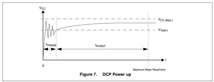
A nonvolatile write to a DCP will change the "wiper position" by simultaneously writing new data to the associated WCR and NVM. Therefore, the new "wiper position" setting is recalled into the WCR after  $V_{\rm CC}$  of the X4023x is powered down and then powered back up.
