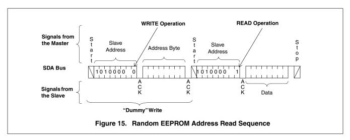
the Device Type Identifier 1010111 or 1010010). Immediately after an operation to a DCP or CR Register is performed, only a "Random EEPROM Read" is available. Immediately following a "Random EEPROM Read", a "Current EEPROM Address Read" or "Sequential EEPROM Read" is once again available (assuming that no access to a DCP or CR Register occur in the interim).
