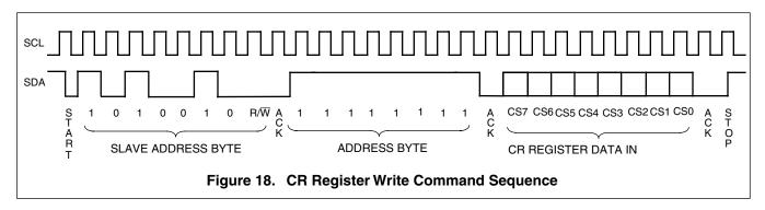
The region of EEPROM memory which is protected / locked is determined by the combination of the BL1 and BL0 bits written to the CR register. It is possible to lock the regions of EEPROM memory shown in the table below:
