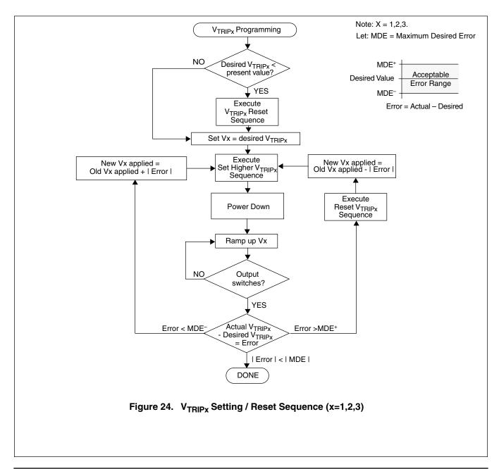
If the calculated error is greater than zero, then the  $V_{TRIPx}$  must first be "reset", and then programmed to the a value equal to the previously set  $V_{TRIPx}$  minus the calculated error. If it is the case that the error is less than zero, then the  $V_{TRIPx}$  must be programmed to a value equal to the previously set  $V_{TRIPx}$  plus the absolute value of the calculated error.
